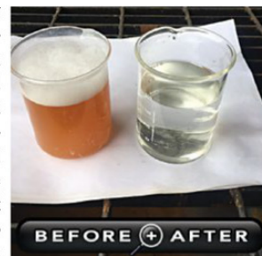
Fig. 5 — Entering and exiting flux.
