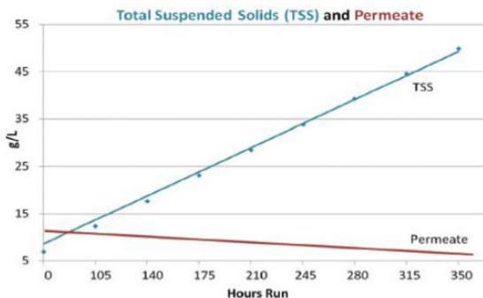
Fig. 9 — Total suspended solids and permeate passing through membrane (Velocity = 10 fps).
