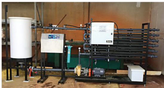
Fig. 6 — Pilot OxyFilter system.
