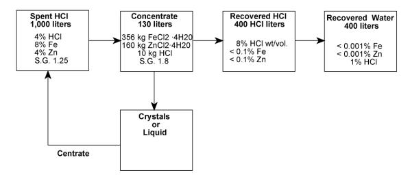
To illustrate the process, we can follow 1,000 liters of a galvanizer's spent pickling acid through the system.
