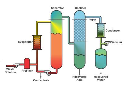
Forced by expansion, the acid and water vapors are driven from the Separator and into the Rectifier. The concentration of acid is controlled in this step to return excellent quality, recovered acid to the process tank.
