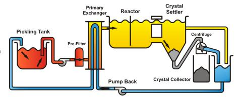
In this heat interchanger the temperature is reduced by using the previously cleaned chilled acid traveling counter-currently through the interchanger. In this way the chilled recovered acid is pre-heated and the hot spent pickle liquor is chilled without using an external energy source. This greatly reduces operating costs.
